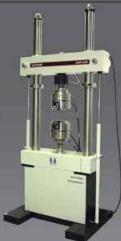
Axial Fatigue Testing Machine 250 kW
