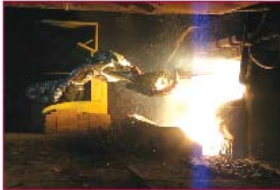
Figure 6: EAF LiquiRob for Temp & Sampling probes
