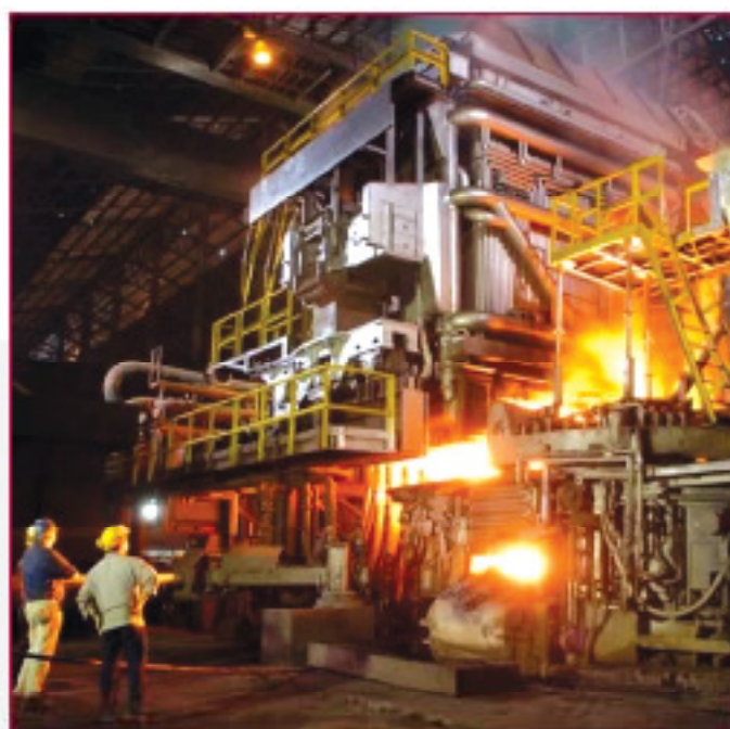
Figure 7: NatSteel finger-shaft electric arc furnace modernized in 2013
