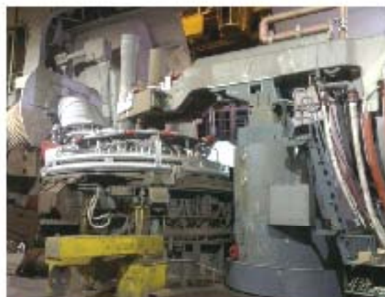
Figure 5: EAF at Swiss Steel, modernized in 2013 with a new furnace gantry, roof, tilting platform, hydraulic system and lad car
