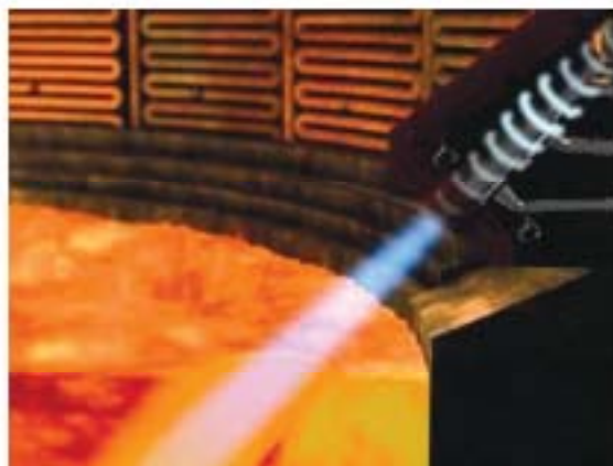
Figure 4: RCB Temp; contact free temperature measurement
