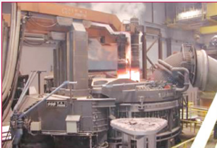
Figure 3: EAF 150t at Outokumpu Stainless
