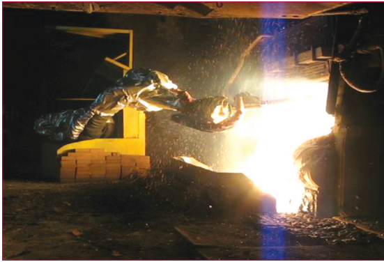
Figure 6: EAF LiquiRob for Temp & Sampling probes
