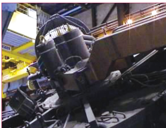
Figure 2: Copper-clad current-conducting electrode arms
