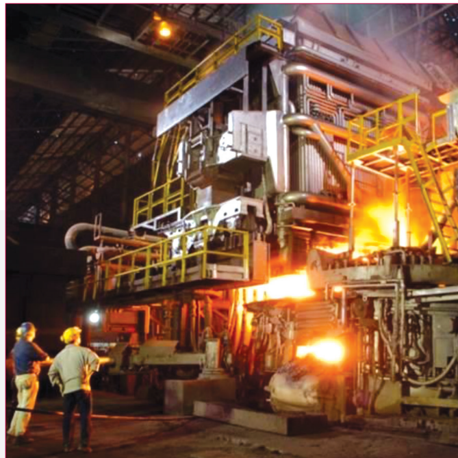
Figure 7: NatSteel finger-shaft electric arc furnace modernized in 2013
